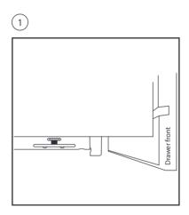
1. Adjust the front of the drawer by rotating the levelling screw, placed under each side of the drawer right behind the front of the drawer.
