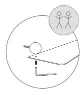
Mount the shelf to the sphere accessory by inserting the small screw beneath the sphere. The shelf should be placed in between the sphere and the screw. Use the small hex key to tighten the screw.
