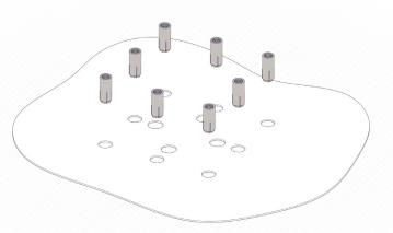
**Step 5.** Hammer to open flange on "Drop in" anchors.
