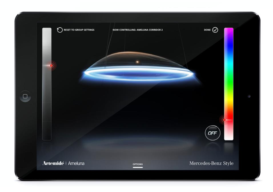
Control the white and rgbw emission by using the lateral bars on the screen, confirm settings tapping "DONE"
