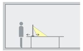
Workplace lighting Lucy task lights with a pedestal can be positioned anywhere in the room. For optimum illumination of the desktop, the luminaire should be placed on the left side for righthanders and on the right for lefthanders.
