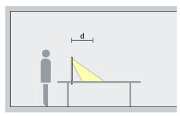
The position of Lucy task lights for desktop mounting depends on the surface to be illuminated. For optimum illumination of the desktop, the luminaire should be placed on the left side for right-handers and on the right for lefthanders. The recommended mounting point is around 40-50cm (a) from the edge of the desk, with a distance (d) of around 50cm to the centre of the beam.
