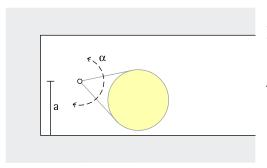
From a single position, the illuminated surface can be adjusted to the area of the visual task thanks to a luminaire head that can be rotated by 180° ( $\alpha$ ).
