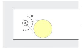
From a single position, the illuminated surface can be adjusted to the area of the visual task thanks to a luminaire head that can be rotated by 180° (α).
