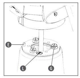
Assemble the type of diffuser on the lamp body ensuring that it corresponds with the reference pin (E) of the diffuser and with the opening (F) present of the lamp body. Insert the head of the three screws (G) into their appropriate slots (H) of the lamp body. Rotate the diffuser clockwise until it locks in position (to turn the diffuser, utilize the external part of the diffuser).
