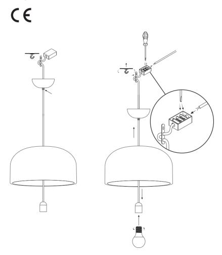
After assembling the wire to the outlet, move the canopy to the ceiling and fasten the relief-screw.
