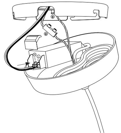
3. Use two fingers to adjust the length of the cord by pushing up or downwards. Roll up the excess cord and place it inside the canopy. Use the large Hex-key included to secure it.
