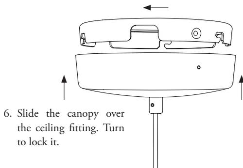
6. Slide the canopy over the ceiling fitting. Turn to lock it.
