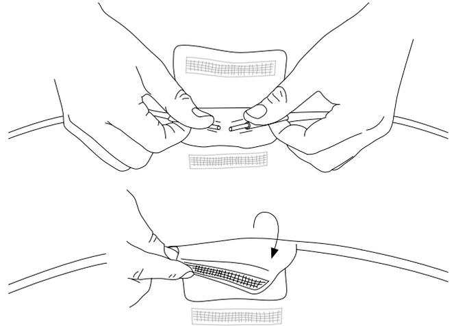
3. Slide the light-bar into the shade and grab it through the hole in middle. Make sure it is centered inside the shade.
