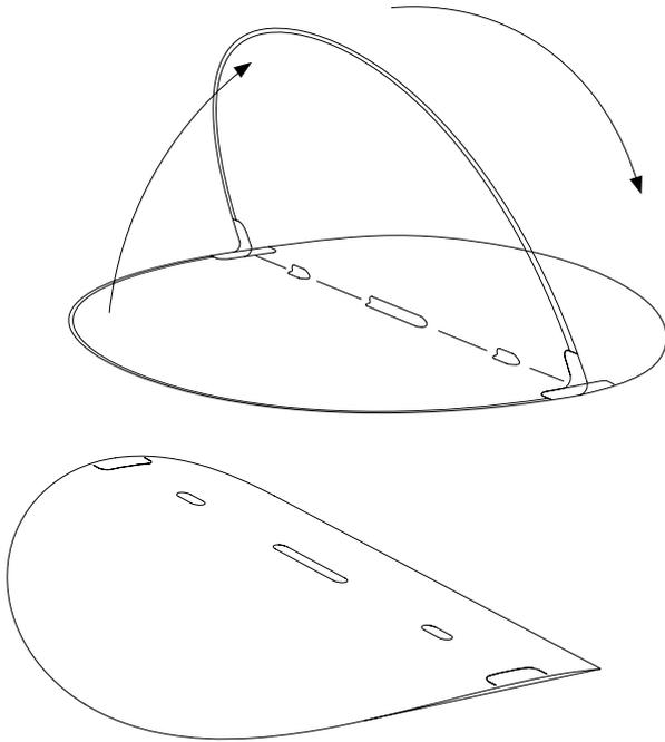
2. Remove the black cap at the end of the rod and push back the black tube, press both ends against each other and slide the tube over the joint to stabilise the frame of the shade. Fold the lid over the joint and inside the hole to close it.
