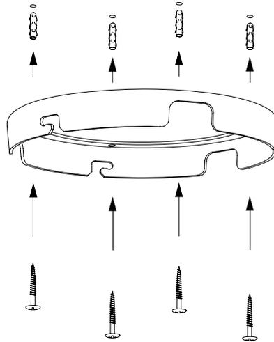
2. Drill holes. Make sure to use plugs and screws appropriate for the ceiling material. Now mount the ceiling fitting.
