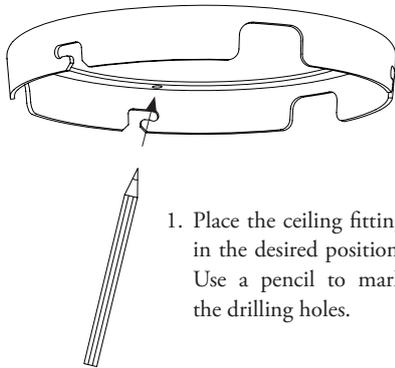
1. Place the ceiling fitting in the desired position. Use a pencil to mark the drilling holes.
