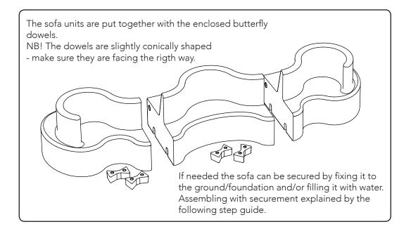
Fix the butterflies at the bottom of the left unit (bolts are enclosed).
