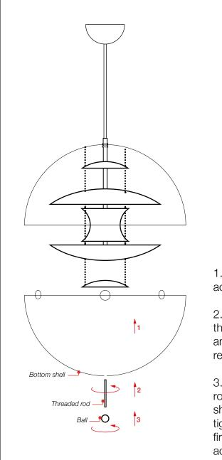
1. Carefully lift the bottom acrylic shell into place.
