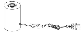
If the external flexible cable or cord of this luminaire is damaged, it shall be exclusively replaced by the manufacturer or his service agent or a similar qualified person in order to avoid a hazard.
