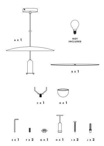
DECIDE THE LENGTH OF THE CORD AND MOUNT THE CEILING ROSE BRACKET USING THE WALL PLUGS AND SCREWS.
