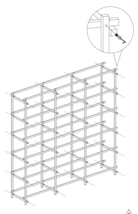
Please ensure all screws are fully tightened before placing the F parts.
