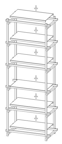
Please ensure all screws are fully tightened before placing the F parts.
