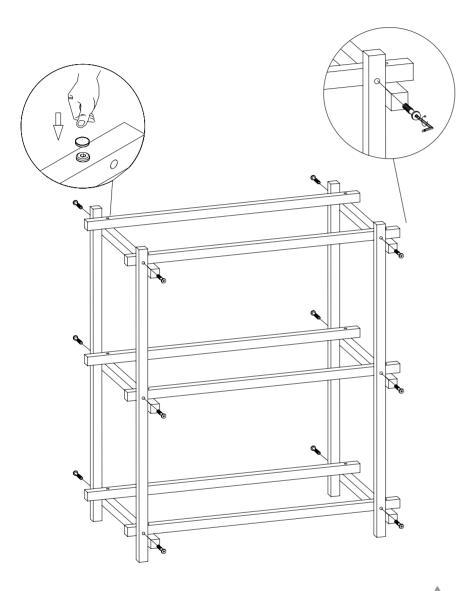
Please ensure all screws are fully tightened before placing the F parts.
