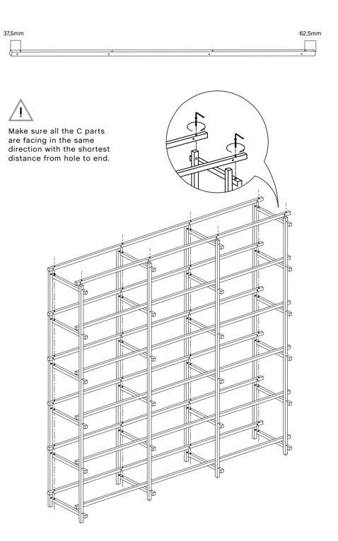
Place the D parts on top of the C parts.
