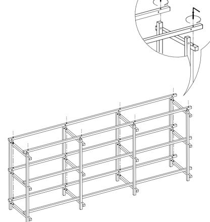
Place the D parts on top of the C parts.
