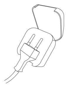
Screw the converter together to ensure the UK plug is secure.
