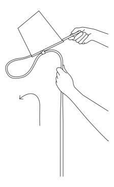
To re-adjust from the up-light position, pull gently on the handle so that the head slides back down the rope.
