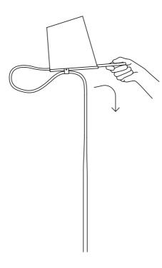
We recommend that you do not extend the head past the minimum and maximum positions shown below (roughly 60 degrees from vertical when sliding back around the loop).
