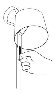
Press the button to switch the light on and off. Press and hold to gradually change the intensity of the light.
