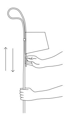
When positioning the head beyond the bend in the rope, hold the upright close to the bend and push the handle gently.
