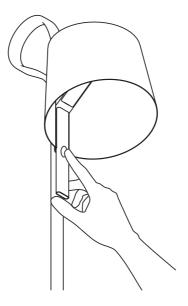
Using one hand to hold the upright and the other on the handle, adjust the height and angle of the head by sliding it around the loop.
