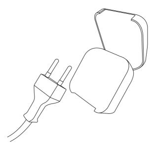
Close the converter over the plug, with the pins secured in the internal clip contacts.
