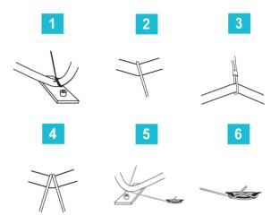
To minimize movement in the table additional tightening of the string can be required. You can easily tighten the strings while the table is in the upright position.
