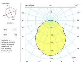
**UTILIZATION: INTERNAL** TYPOLOGY: HANGING **COLOURS** STRUCTURE: WHITE DIFFUSER: **SATIN WHITE** STRUCTURE: **ALUMINIUM MATERIALS** DIFFUSER: **METHACRYLATE MEASURES** WIDTH: -DIAMETER: 41 cm WEIGHT NET: 3,5 HEIGHT: 16 cm HOLE DIAMETER: -GROSS: -HOLE DEPTH: -LENGTH: -DEPTH: -PACKAGING VOL.M3: -NUMBER OF ITEMS: 1 BULBS LED 1X13W
