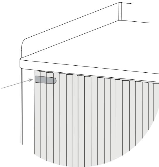
Wheel must always be on the bottom of the door
