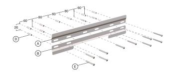
Slide the shelf  $\bigcirc$  onto the mounting bracket  $\bigcirc$  and  $\bigcirc$  .
