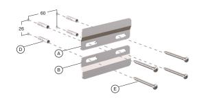
Slide the shelf © onto the mounting brackets (A) and (B).
