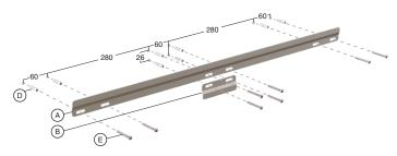
Slide the shelf © onto the mounting bracket A and B.
