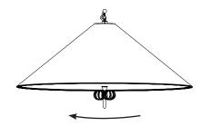
Turn the center handle to secure the diffuser to the lamp.
