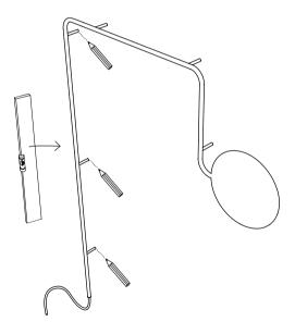
MOUNT THE WALL LIGHT ONTO THE SCREWS ON THE WALL
