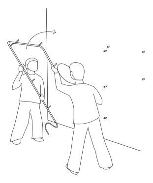
APPLY THE SMALL LOCK SCREWS TO MOUNT THE WALL LIGHT ONTO THE SCREWS IN THE WALL
