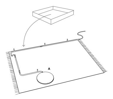
PULL THE CORD TO CONNECT THE TUBULAR METAL FRAME. MAKE SURE TO ALIGN THE TUBES BEFORE APPLYING THE LOCK SCREWS WITH THE HEX KEY. MOUNT THE SHADE TO PIPE WITH THE M4 SCREW.
