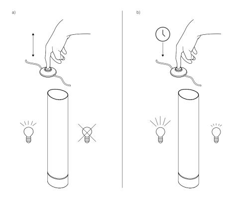
Push the switch once to turn on. (a) Push again to turn off. (b)
