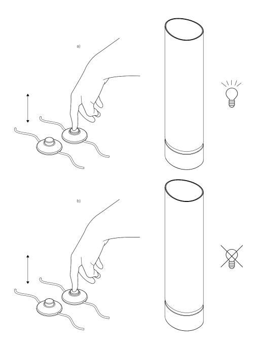
Hold the switch to increase light intensity. (a) Hold the switch again to decrease light intensity. (b)
