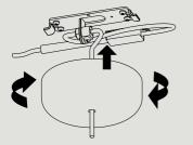
Step 5 Install the plastic canopy onto the metal bracket
